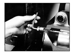
Turn adjusting screw assembly into housing
